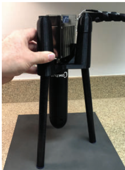
▲ Fig. 4 Integrated 2 to 18 GHz reflectometer system including both sensor and vector analyzer.
