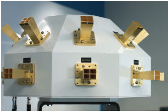
▲ Fig. 10 28 GHz Channel sounder by AT&T and National Instruments (courtesy National Instruments).
