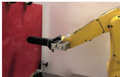
▲ Fig. 6 Robot arm with spot probe and vector analyzer scanning a fiberglass panel.
