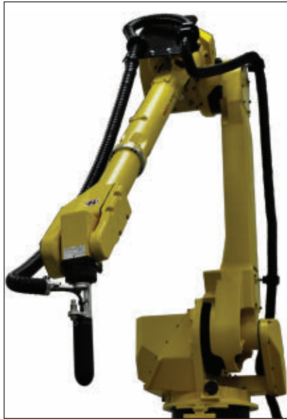
▲ Fig. 1 Robotic arm with microwave probe sensor and flexible RF cable along the arm.
